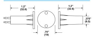
For mounting drill 3/8"(10 mm) hole (Dimensions in brackets are in mm)
