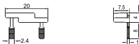
S1D-B1, 10A @ 250 VAC, 1 Way Bridge for Coil
