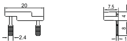
S1D-B1, 10A @ 250 VAC, 1 Way Bridge for Coil
